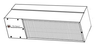
("B") Remove Cover Plate and Grill Remove Pilot Screen if applicable (2 screws)
